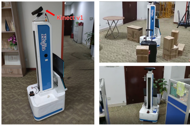
Fig. 5. Our mobile robot platform (left). A testing environment with static obstacles (upper right) and an office scenario (bottom right).
