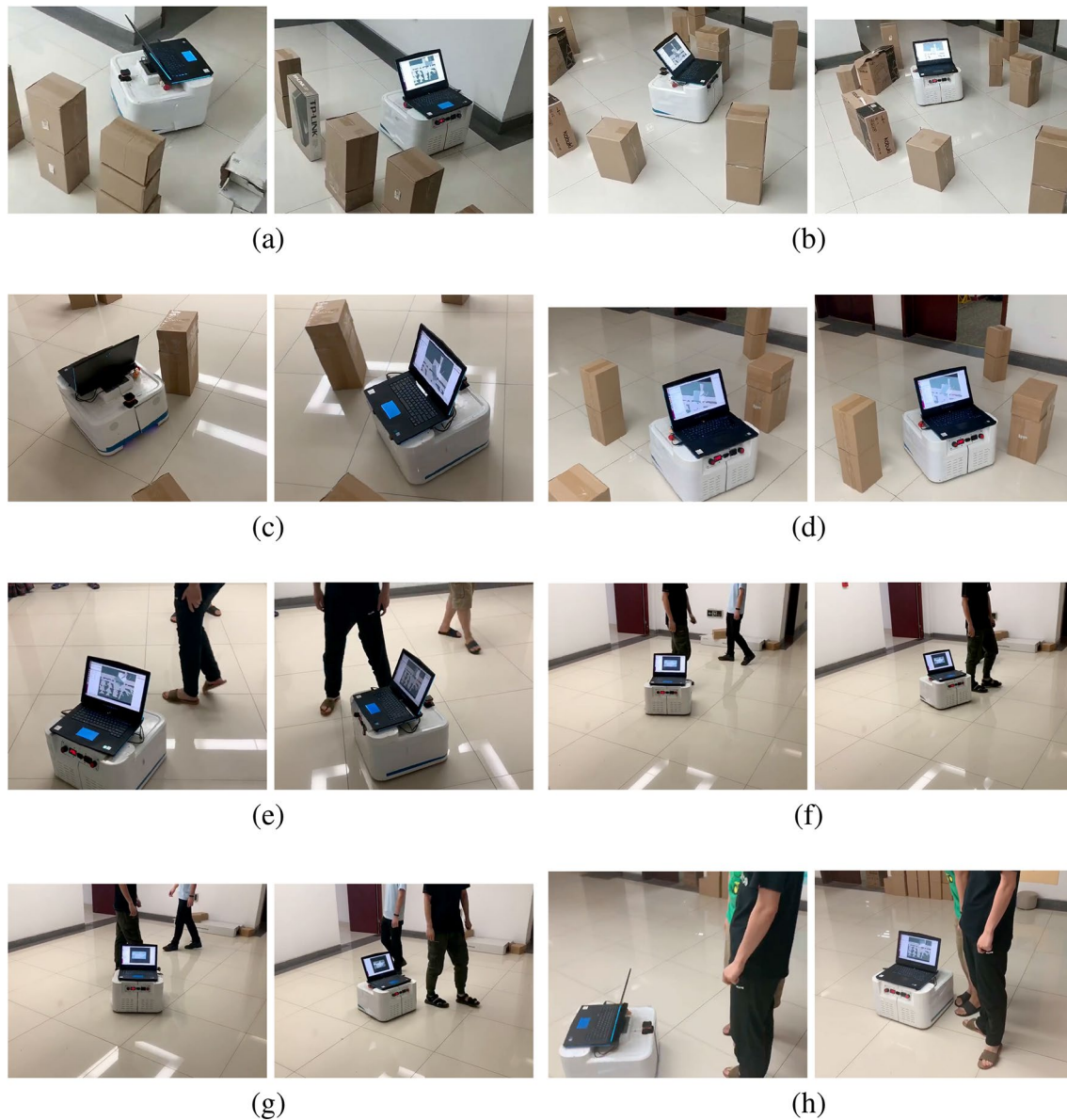
Fig. 12 Robot test of obstacle avoidance module, including right-angle (a) and s-shaped environment (b), discrete random obstacles environment (c, d). And the robot successfully avoided passing pedestrians (e, f, g) and sudden still pedestrians (h)
