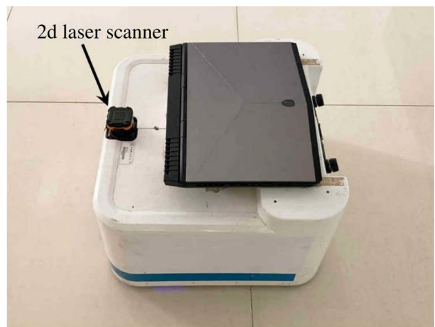
Fig. 11 Our robot chassis with a laptop and a Hokuyo UTM-30LX laser scanner
