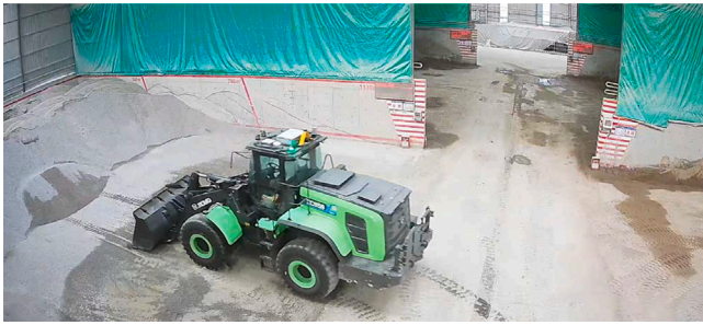
Fig. 25. Field deployment of the autonomous shoveling system on a new XCMG XC958EV wheel loader at a mixing station in Shandong, China.
